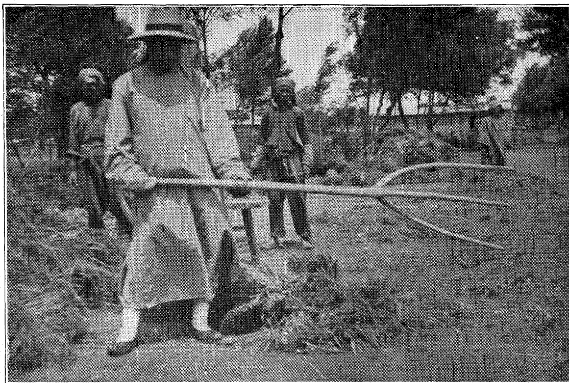
Fig. 46.—Wooden fork shaped from the limbs of a tree by simple means of steaming and drying.
